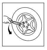
Loosen all five hex-shaped plastic caps by turning the wheel wrench counterclockwise.
